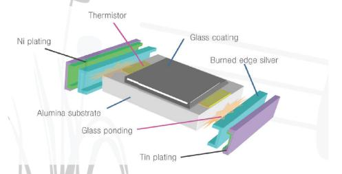
corrosive gases, like e.g. sulphur as well as against moisture. The further advantage of these thick film sensors lays in the variable adjustment of the  $R_{25}$  – (100  $\Omega$  to 2 M $\Omega$ ) and B values (2700 – 5000 K) as well as in the corresponding tolerances ( $\pm$  1 to  $\pm$  10 %), which is possible due to Tateyama's patented manufacturing technology.
