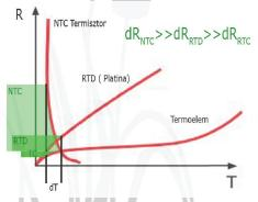
resistance value of  $100\Omega$  at  $0^{\circ}$ C. The main disadvantage of this type of device is the cost, platinum is an expensive material.
